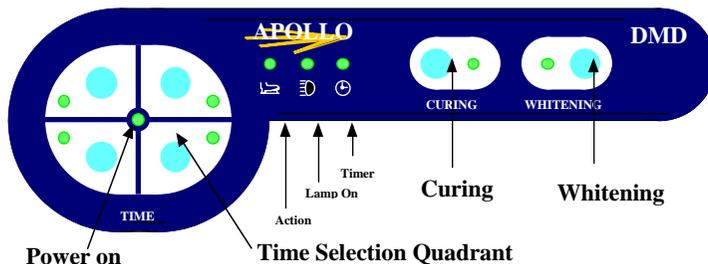
Variation in line voltage has no effect on the lamp intensity. The exposition time can be selected for 1 second, 2 seconds, 3 seconds or SC (step curing: 2 seconds at half power, followed by 4 seconds at full power).
